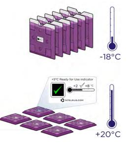
**3.** The Utektile panels define a fixed payload space where temperature control is maintained. Place one panel in the base of the ORCA insulation, with front label facing upwards then arrange four other panels around the vertical walls of the insulation with the labelled faces inwards. The payload can now be inserted into the space defined by these 5 panels. The remaining panel can now be added to the top with the label facing downwards.
