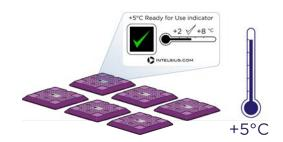
The Utektile panels define a fixed payload space where temperature control is maintained. Place one panel in the base of the ORCA insulation, with front label facing upwards then arrange four other panels around the vertical walls of the insulation with the labelled faces inwards. The payload can now be inserted into the space defined by these 5 panels. The remaining panel can now be added to the top with the label facing downwards.
