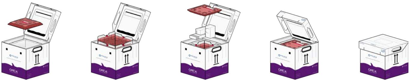
**4.** Close the outer carton lid, secure the fasteners and seal with two strips of packing tape following the tape area marked with dotted lines. The ORCA is now ready to be shipped.
