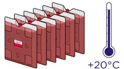
**3.** The Utektile panels define a fixed payload space where temperature control is maintained. Place one panel in the base of the ORCA insulation, with front label facing upwards then arrange four other panels around the vertical walls of the insulation with the labelled faces inwards. The payload can now be inserted into the space defined by these 5 panels. The remaining panel can now be added to the top with the label facing downwards.
